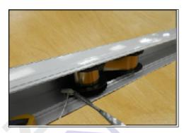
Clamp the string at the spring location to stop tension. A second person can secure the string if a clamp tool is unavailable.
