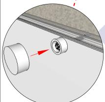
Note - For shades over 96" wide, install the flap support screw in the center of the width of the pocket, 1/8" down from the top of the pocket (through the pocket and into the flap) to support the center. It is important that the screw is no more than 1/8" down from the top and 1.5" long so that it does not damage the fabric. Then snap on the cap to conceal it.
